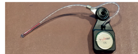
Fevertag - a device used for monitoring fever in calves, which sits in the ear canal.
